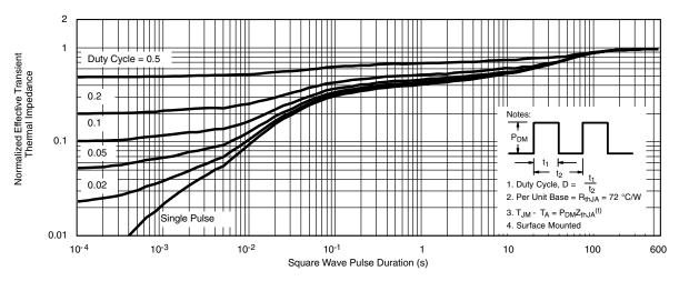
Normalized Thermal Transient Impedance, Junction-to-Ambient
