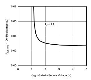
On-Resistance vs. Gate-to-Source Voltage
