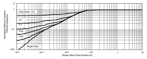
Normalized Thermal Transient Impedance, Junction-to-Foot
