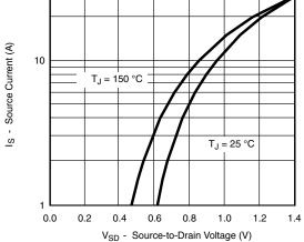
Source-Drain Diode Forward Voltage
