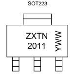
ZXTN 2011 = Product Type Marking Code YWW = Date Code Marking Y or  $\overline{Y}$  = Last Digit of Year (ex: 5= 2015) WW or  $\overline{W}W$  = Week Code (01~53)
