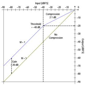
Figure 17. Audio Dynamic Range Transfer Function
