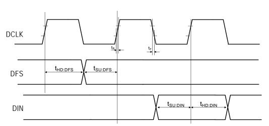
Figure 8. Digital Audio Interface Timing Parameters, I<sup>2</sup>S Mode
