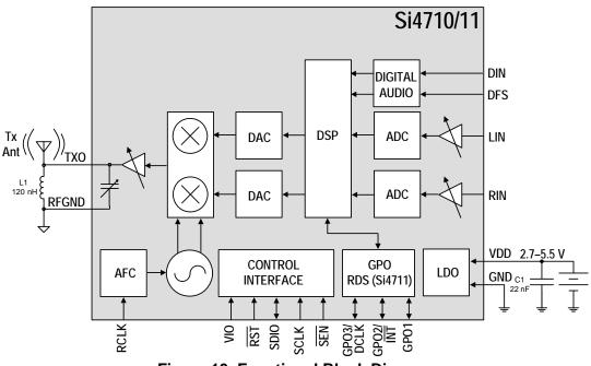
Figure 13. Functional Block Diagram
