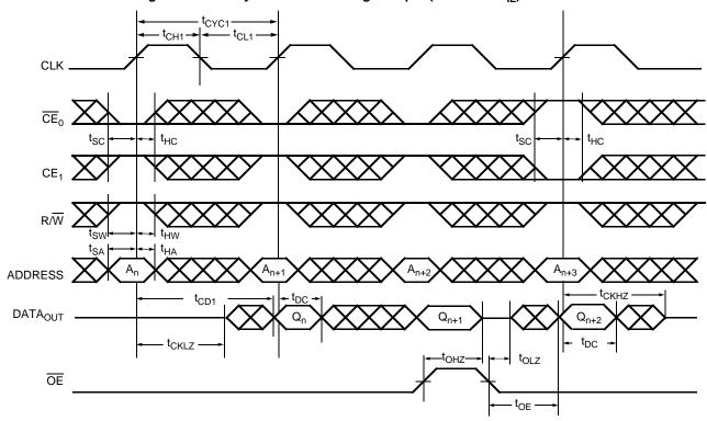
Figure 3. Read Cycle for Pipelined Operation ( $\overline{\text{FT}}/\text{PIPE} = V_{\text{IH}})^{[5, \, 6, \, 7, \, 8]}$
