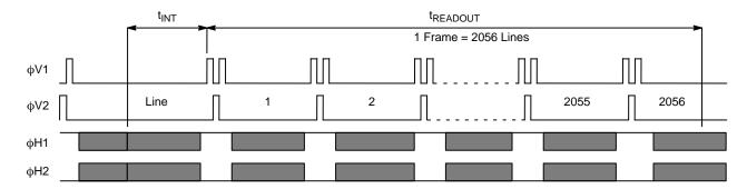
Figure 7. Frame Timing
