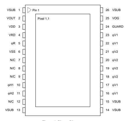
Figure 4. Pinout Diagram
