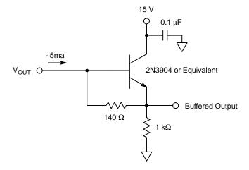
Figure 3. Typical Output Structure Load Diagram
