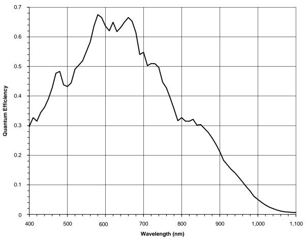
Figure 5. Typical Spectral Response
