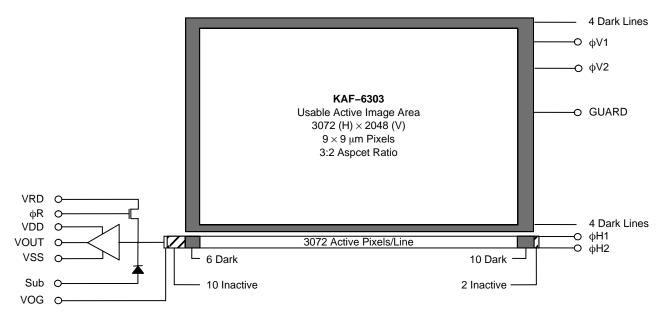
Figure 2. Block Diagram
