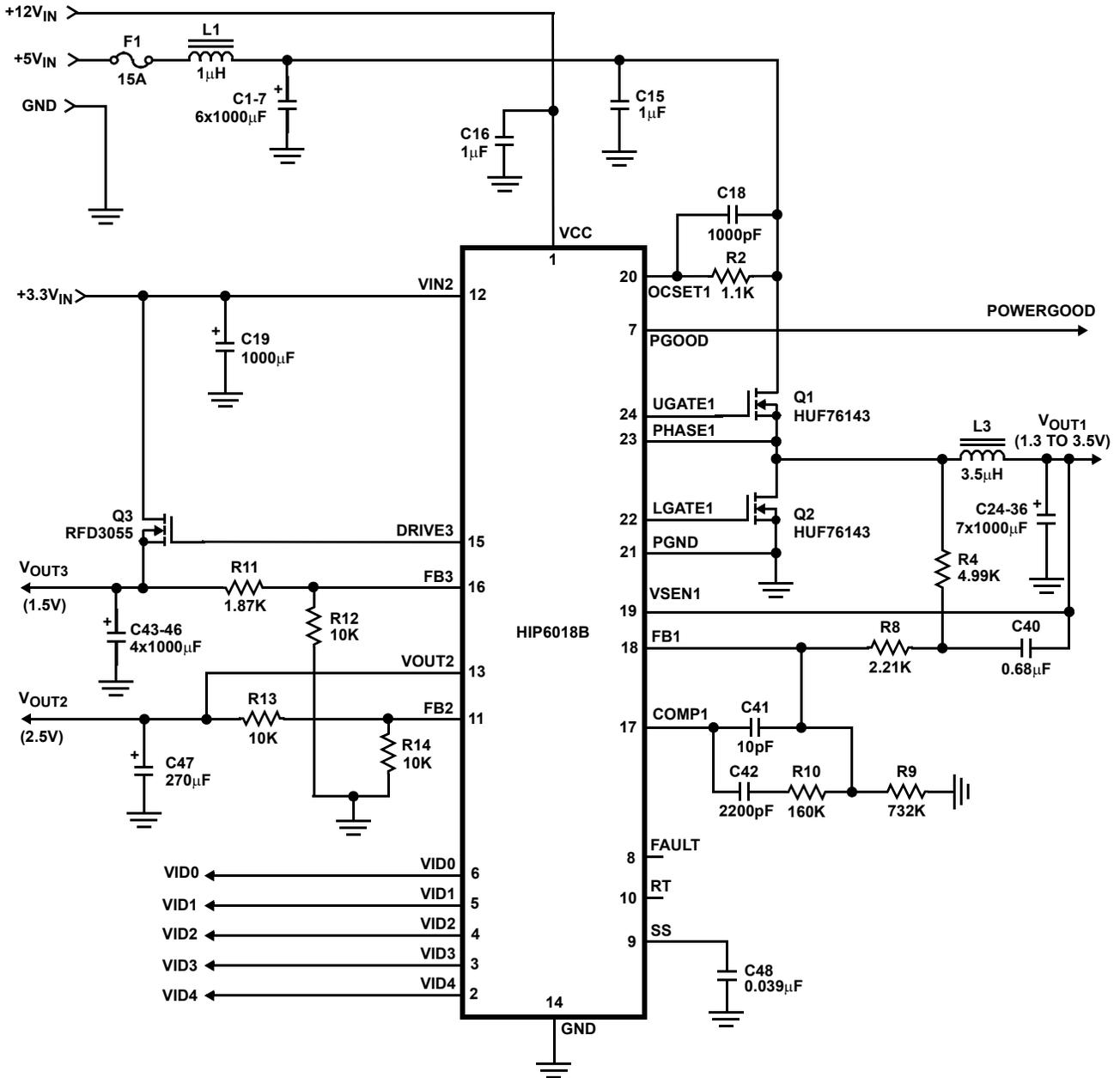
FIGURE 15. APPLICATION CIRCUIT
