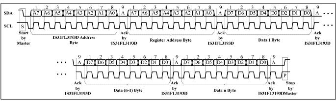
Figure 5 Writing to IS31FL3193D (Automatic Address Increment)
