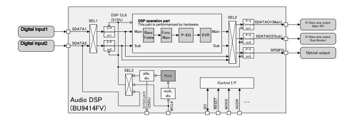
BU9414FV has 2 digital stereo input and 3 digital stereo output with the same sampling rate.
