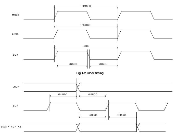
Fig 1-3 Audio interface timing
