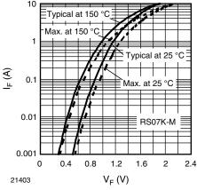
Fig. 2 - Typical Forward Characteristics
