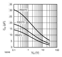
Fig. 4 - Typical Diode Capacitance vs. Reverse Voltage
