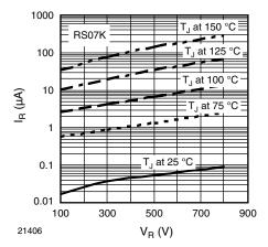
Fig. 7 - Typical Reverse Characteristics
