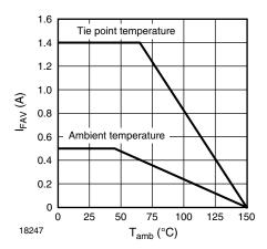
Fig. 3 - Forward Current Derating Curve
