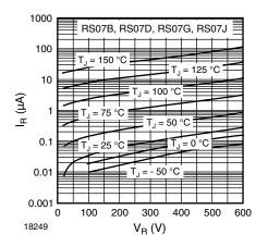
Fig. 6 - Typical Reverse Characteristics
