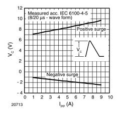
Fig. 6 - Typical Clamping Voltage vs. Peak Pulse Current I<sub>PP</sub>
