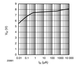
Fig. 5 - Typical Reverse Voltage  $V_{\text{R}}$  vs. Reverse Current  $I_{\text{R}}$
