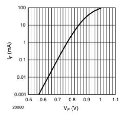
Fig. 4 - Typical Forward Current I<sub>F</sub> vs. Forward Voltage V<sub>F</sub>
