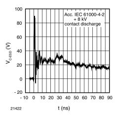
Fig. 9 - Typical Clamping Performance at + 8 kV Contact Discharge (acc. IEC 61000-4-2)
