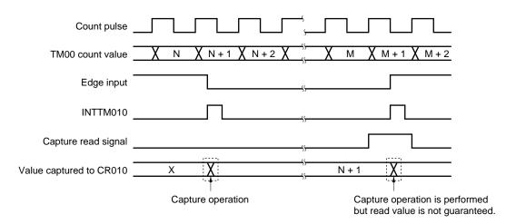
Figure 7-57. Timing of Holding Data by Capture Register
