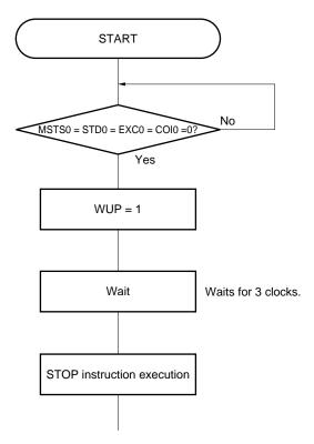
Figure 15-23. Flow When Setting WUP = 1
