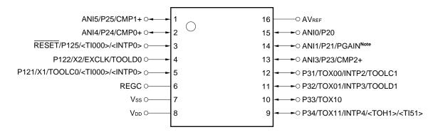
PGAIN Note: Programmable Gain REGC: Regulator Capacitance
