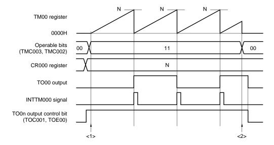
Figure 7-19. Example of Software Processing for Square-Wave Output Function
