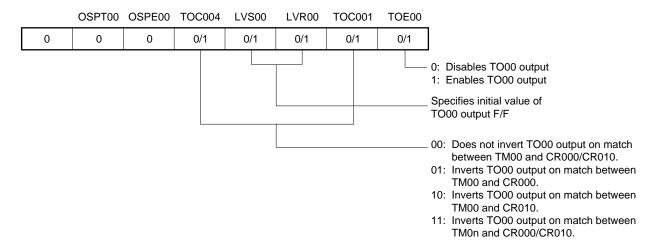
Figure 7-39. Example of Register Settings in Free-Running Timer Mode (2/2)
