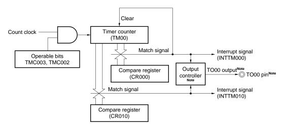
Figure 7-41. Block Diagram of PPG Output Operation
