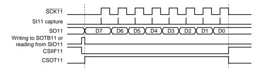
Remark The above figure illustrates a communication operation where data is transmitted with the MSB first.
