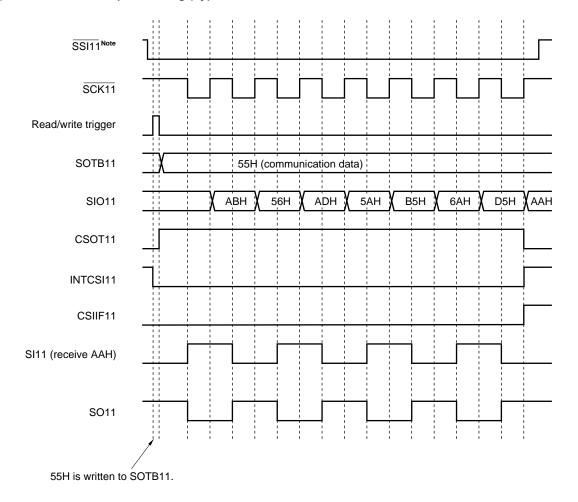
**Note** The SSE11 flag and  $\overline{SSI11}$  pins are used in the slave mode.
