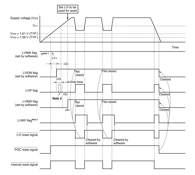
Figure 22-4. Timing of Low-Voltage Detector Internal Reset Signal Generation (LVISTART = 0)
