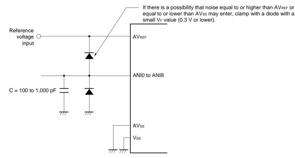
Figure 11-25. Analog Input Pin Connection
