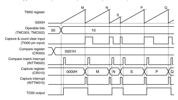
This is an application example where the TO00 output level is inverted when the count value has been captured & cleared.
