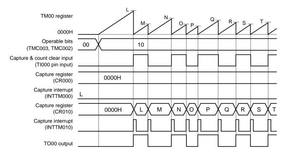
This is an application example where the count value is captured to CR010, TM00 is cleared, and the TO00 output is inverted when the rising or falling edge of the Tl000 pin is detected.
