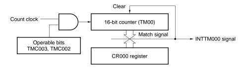
Figure 7-13. Basic Timing Example of Interval Timer Operation
