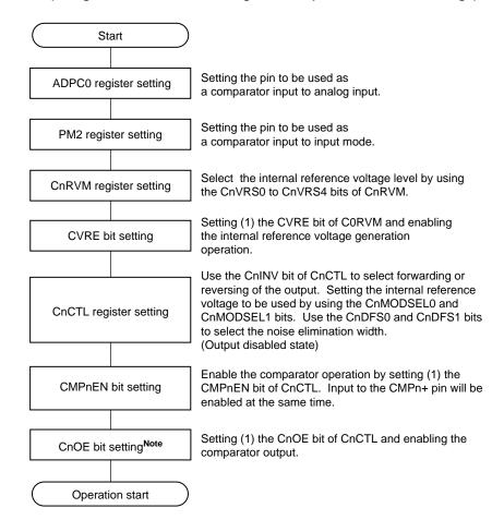
**Note** Set the CnOE bit to 1 when at least 20  $\mu$  s have elapsed after having set the CVRE register.
