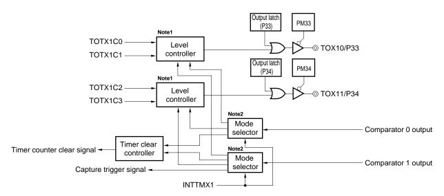
Figure 6-44. Block Diagram of 16-Bit Timer X1 Output Configuration
