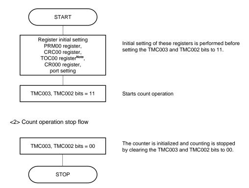
Note Care must be exercised when setting TOC00. For details, refer to 7.3 (3) 16-bit timer output control register 00 (TOC00).
