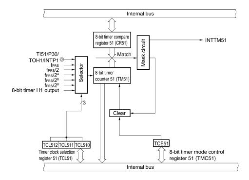
Figure 8-1. Block Diagram of 8-Bit Timer/Event Counter 51
