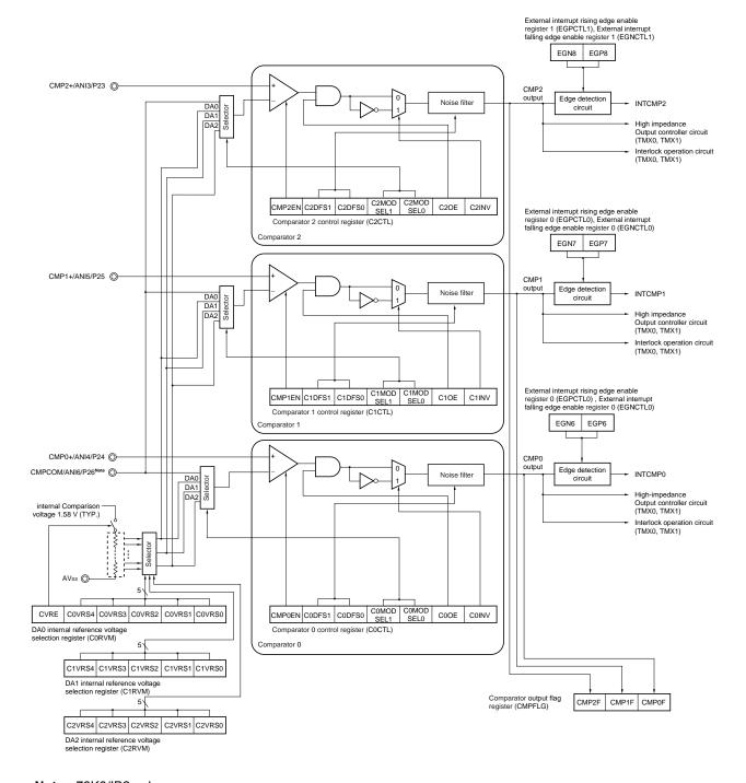
Figure 13-1. Block Diagram of Comparators
