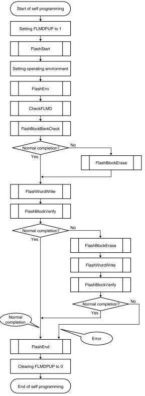
Figure 25-9. Flow of Self Programming (Rewriting Flash Memory)
