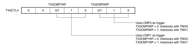
**Remark** When interlocking the timers with either CMP0 or CMP1, set all bits of CMP0 or CMP1, whichever is not used, to 0.
