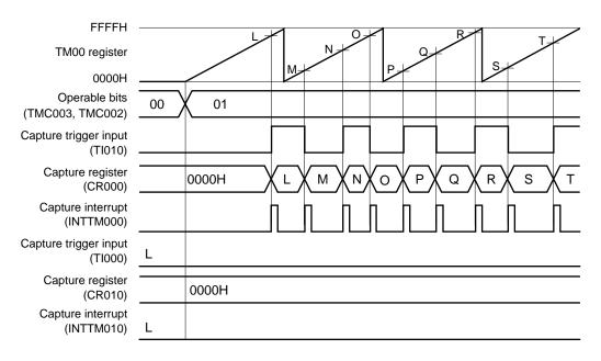
This is an application example where both the edges of the Tl010 pin are detected and the count value is captured to CR000 in the free-running timer mode.
