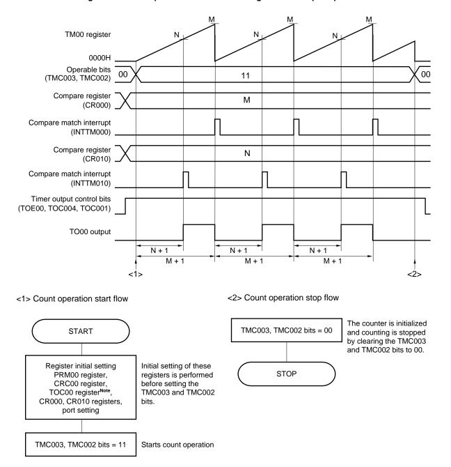
Figure 7-43. Example of Software Processing for PPG Output Operation
