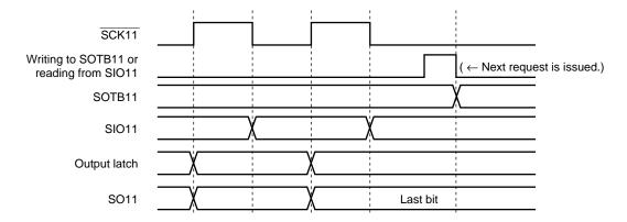
Figure 16-9. Output Value of SO11 Pin (Last Bit) (2/2)
