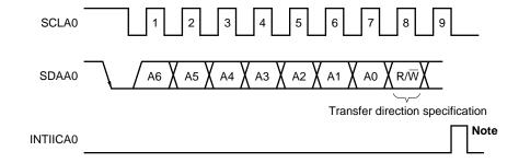
**Note** INTIICA0 is not issued if data other than a local address or extension code is received during slave device operation.
