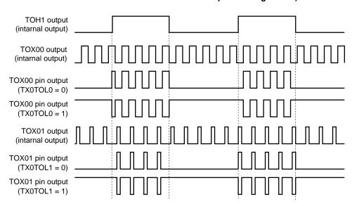
Figure 6-36. PWM Output Timing (TMX0-Only Operation (Dual Output), PWM Output from TOX00 and TOX01 When TOH1 Output Is at High Level)
