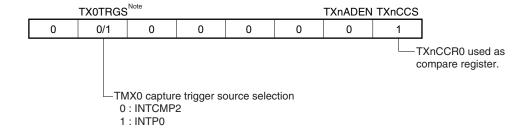
Note The TX0TRGS bit is not provided in the TX1CTL2 register.
