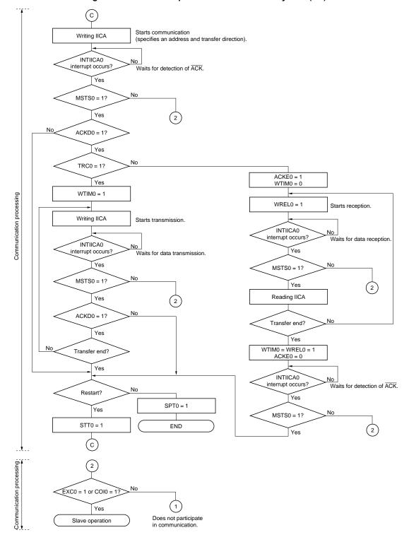
Figure 15-30. Master Operation in Multi-Master System (3/3)
