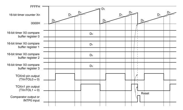
Figure 6-49. Timing of Interlocking mode 2 (timer restart mode)
