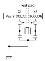
Figure 25-5. Example of Mounting Test Pads
