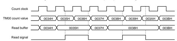
Figure 7-59. 16-bit Timer Counter 00 (TM00) Read Timing
