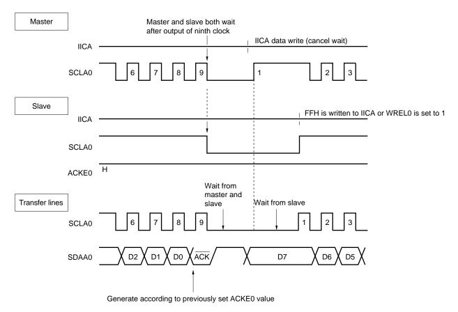
Remark ACKE0: Bit 2 of IICA control register 0 (IICACTL0)
