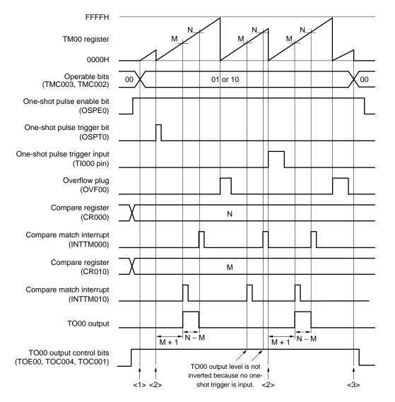
Figure 7-46. Example of Software Processing for One-Shot Pulse Output Operation (1/2)
