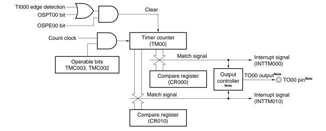
Figure 7-44. Block Diagram of One-Shot Pulse Output Operation
