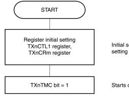
Initial setting of these registers is performed before setting the TXnTMC bit to 1.
