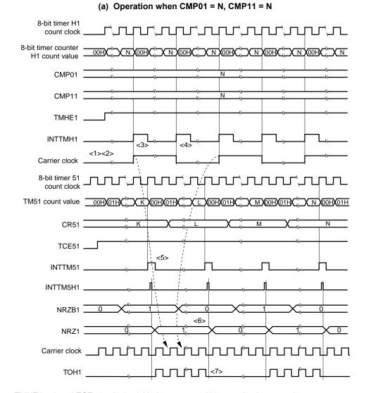
Figure 9-15. Carrier Generator Mode Operation Timing (1/3)
