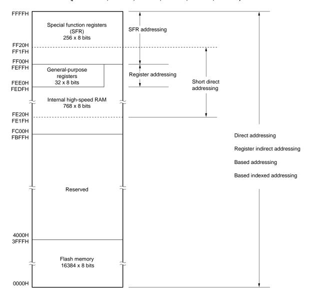
Figure 3-6. Correspondence Between Data Memory and Addressing  $(\mu PD78F0742, 78F0744, 78F0746, 78F0752, 78F0754, 78F0756)$
