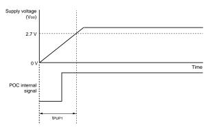
When RESET pin input is used (when external reset is released by the RESET pin, after POC has been released)
