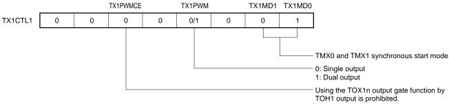
Figure 6-31. Example of Register Settings for PWM Output Operation (TMX0 and TMX1 Synchronous Start Mode) (2/2)
