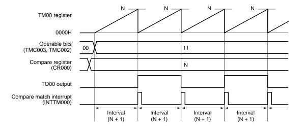
Figure 7-17. Basic Timing Example of Square-Wave Output Operation
