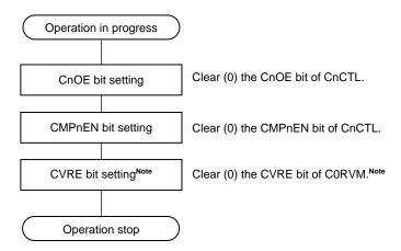
**Note** Only when using the internal reference voltage.
