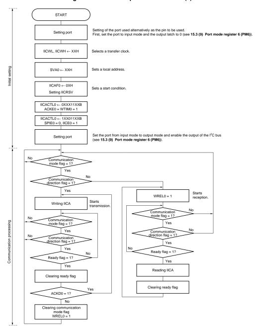
Figure 15-31. Slave Operation Flowchart (1)
