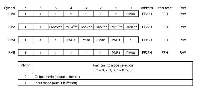
Note If this pin is set as an analog input by using the ADPC0 register, be sure to set it to input mode.
