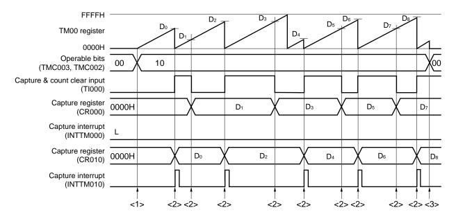
Figure 7-53. Example of Software Processing for Pulse Width Measurement (2/2)
