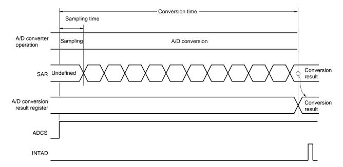
A/D conversion operations are performed continuously until bit 7 (ADCS) of the A/D converter mode register 0 (ADM0) is reset (0) by software.
