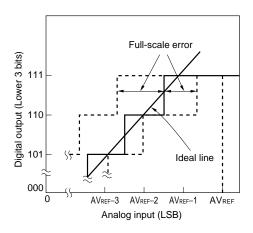
Figure 11-24. Differential Linearity Error
