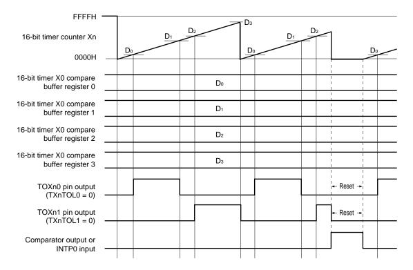
Figure 6-47. Timing of Interlocking mode 1 (timer reset mode)
