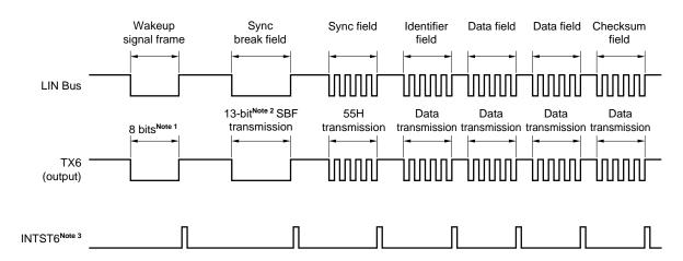
Figure 14-1. LIN Transmission Operation
