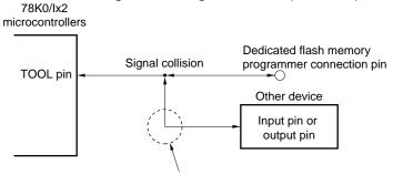
In the flash memory programming mode, the signal of the other device collides with the signal of the dedicated flash programmer. Therefore, isolate the signal of the other device.
