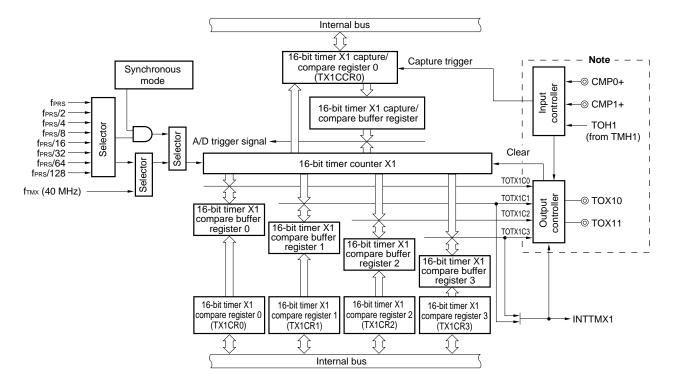
Figure 6-2. Block Diagram of 16-Bit Timer X1
