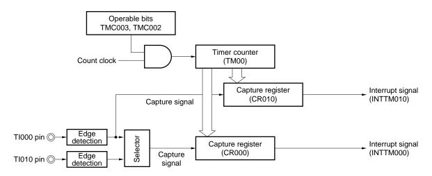
Figure 7-48. Block Diagram of Pulse Width Measurement (Clear & Start Mode Entered by Tl000 Pin Valid Edge Input)
