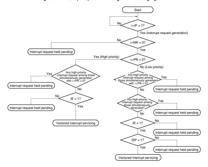
Figure 18-14. Interrupt Request Acknowledgment Processing Algorithm
