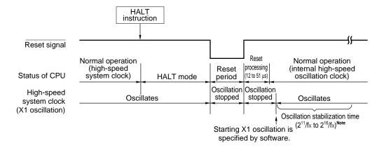
**Note** Oscillation stabilization time is not required when using the external main system clock (fexclk) as the high-speed system clock.
