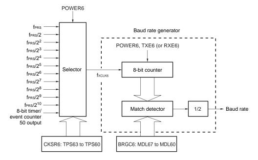
Figure 14-34. Configuration of Baud Rate Generator
