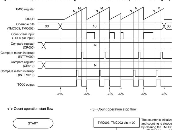
Figure 7-32. Example of Software Processing in Clear & Start Mode Entered by TI000 Pin Valid Edge Input
