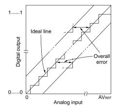
Figure 11-20. Quantization Error
