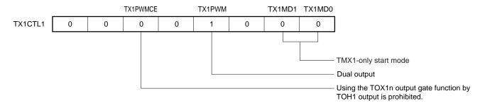
Figure 6-29. Example of Register Settings for PWM Output Operation (Dual Mode) (2/2)
