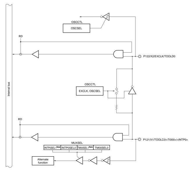
Figure 4-23. Block Diagram of P121, P122
