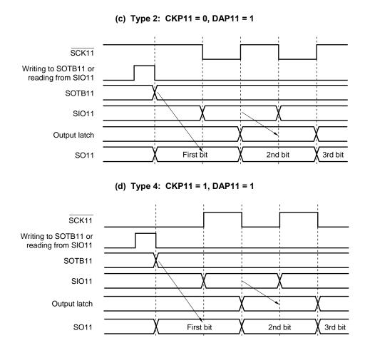
Figure 16-8. Output Operation of First Bit (2/2)
