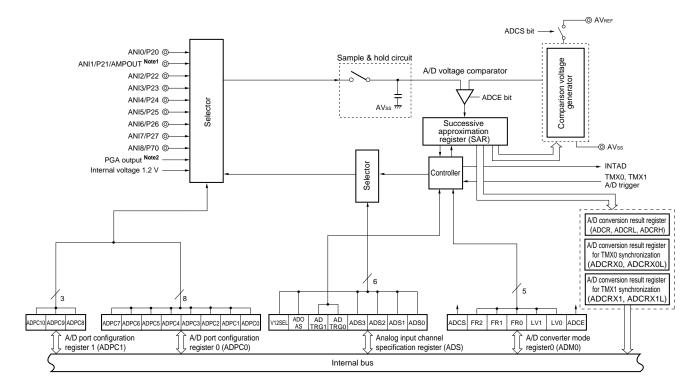
Figure 11-1. Block Diagram of A/D Converter
