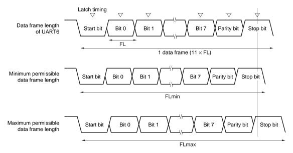
As shown in Figure 14-35, the latch timing of the receive data is determined by the counter set by baud rate generator control register 6 (BRGC6) after the start bit has been detected. If the last data (stop bit) meets this latch timing, the data can be correctly received.
