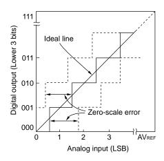
Figure 11-23. Integral Linearity Error
