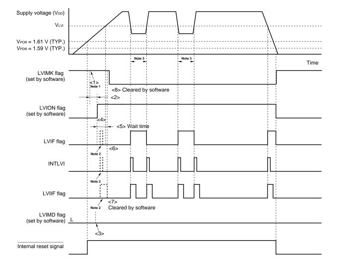
Figure 22-6. Timing of Low-Voltage Detector Interrupt Signal Generation (LVISTART = 0)
