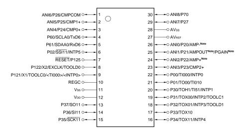
AMP-Note, AMP+Note: Amplifier Input REGC: Regulator Capacitance
