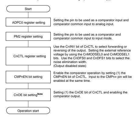
**Note** Set the CnOE bit to 1 when at least 1  $\mu$  s have elapsed after having set the CMPnEN bit.
