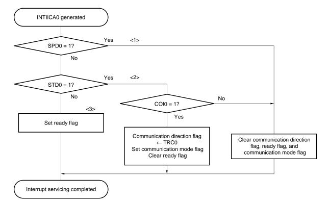
Figure 15-32. Slave Operation Flowchart (2)
