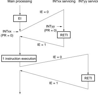
Figure 18-17. Examples of Multiple Interrupt Servicing (2/2)
