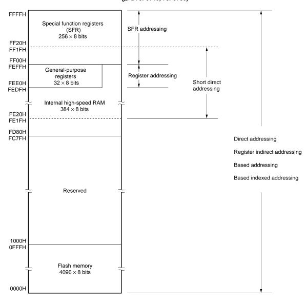
Figure 3-4. Correspondence Between Data Memory and Addressing (μPD78F0740, 78F0750)
