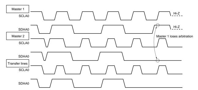
Figure 15-22. Arbitration Timing Example
