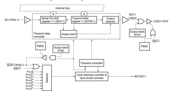
Figure 16-1. Block Diagram of Serial Interface CSI11
