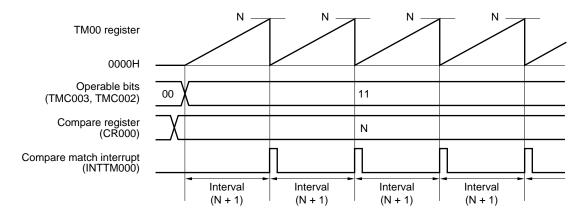
Figure 7-14. Example of Register Settings for Interval Timer Operation
