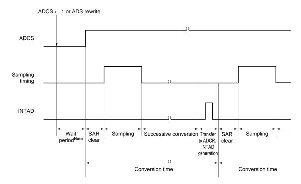
Figure 11-4. A/D Converter Sampling and A/D Conversion Timing
