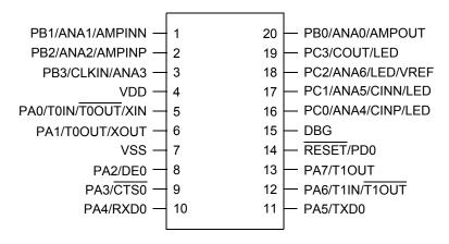
Figure 3. Z8F08xA, Z8F04xA, Z8F02xA, and Z8F01xA in 20-Pin SOIC, SSOP or PDIP Package
