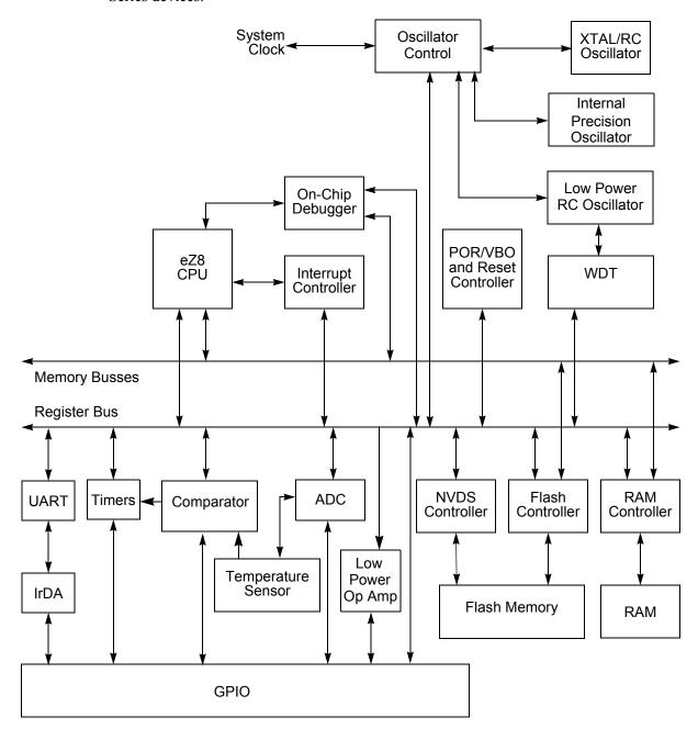
Figure 1. Z8 Encore! XP F082A Series Block Diagram
