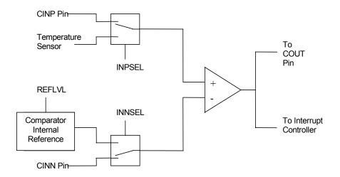
Figure 20. Comparator Block Diagram
