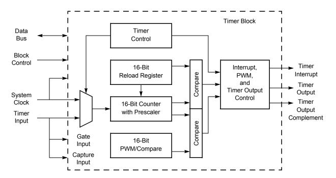
Figure 9. Timer Block Diagram
