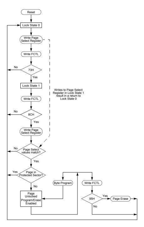
Figure 22. Flash Controller Operation Flow Chart
