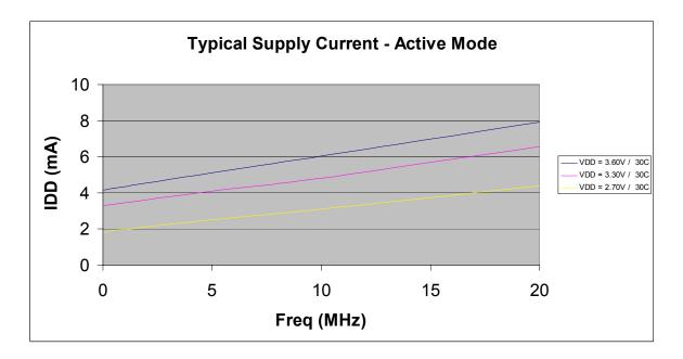
Figure 33. Typical Active Mode I<sub>DD</sub> Versus System Clock Frequency
