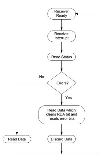
Figure 15. UART Receiver Interrupt Service Routine Flow
