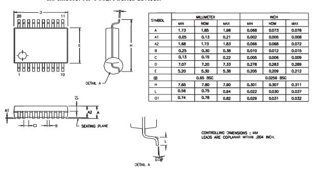
Figure 44. 20-Pin Small Shrink Outline Package (SSOP)
