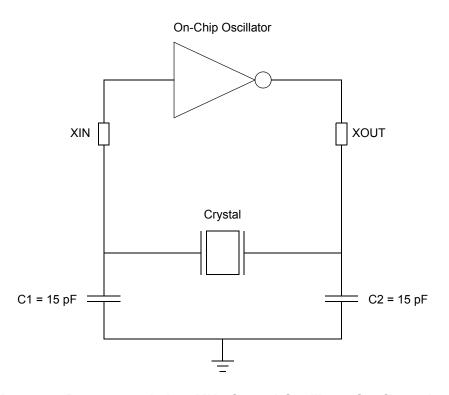
Figure 27. Recommended 20 MHz Crystal Oscillator Configuration
