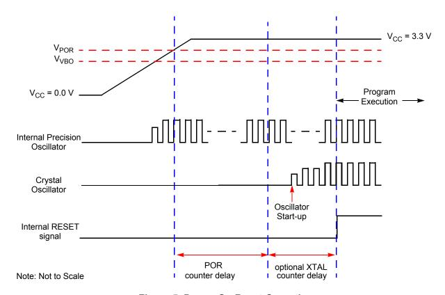
Figure 5. Power-On Reset Operation
