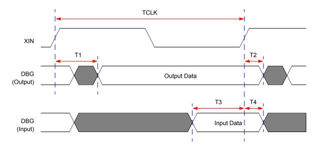
Figure 36. On-Chip Debugger Timing
