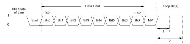
Figure 13. UART Asynchronous MULTIPROCESSOR Mode Data Format
