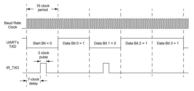
Figure 17. Infrared Data Transmission
