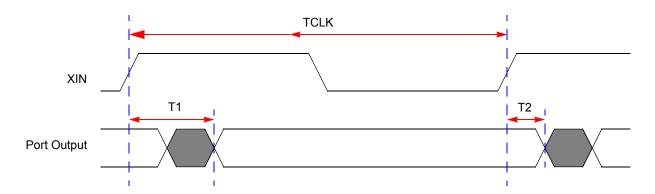
**Figure 35. GPIO Port Output Timing**
