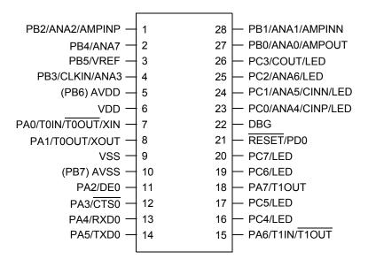
Figure 4. Z8F08xA, Z8F04xA, Z8F02xA, and Z8F01xA in 28-Pin SOIC, SSOP or PDIP Package
