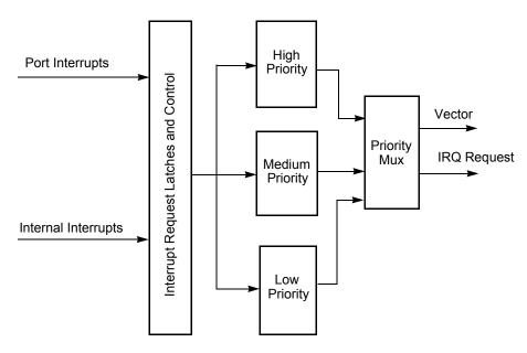
Figure 8. Interrupt Controller Block Diagram
