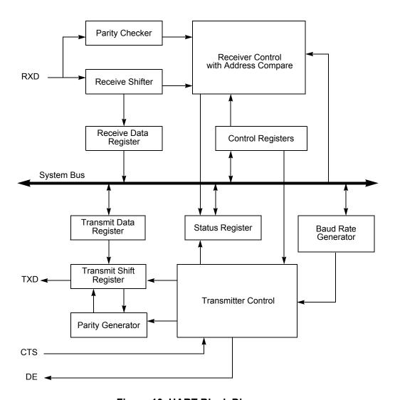
Figure 10. UART Block Diagram
