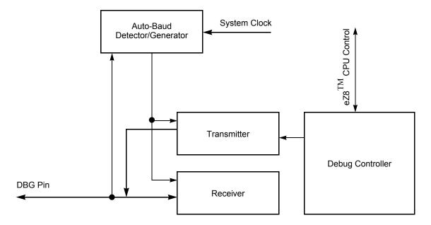
Figure 23. On-Chip Debugger Block Diagram
