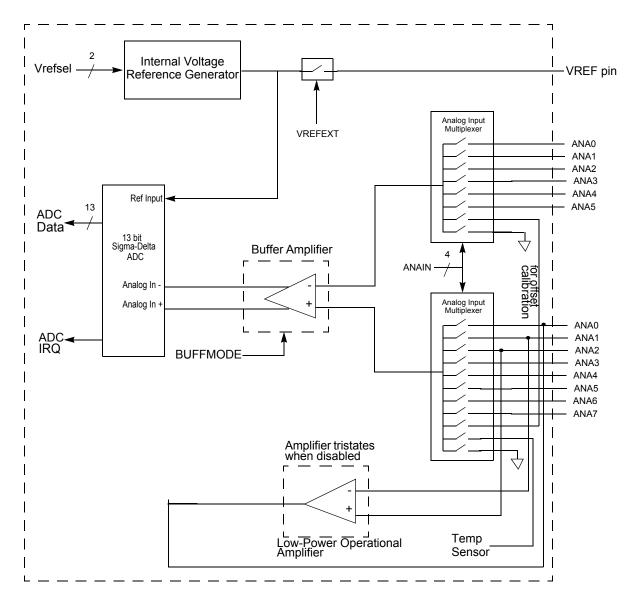
Figure 19. Analog-to-Digital Converter Block Diagram
