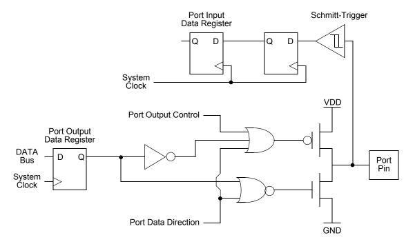
Figure 7. GPIO Port Pin Block Diagram
