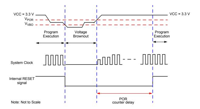
Figure 6. Voltage Brownout Reset Operation
