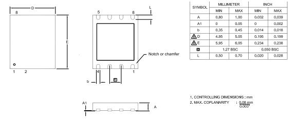
Figure 41. 8-Pin Quad Flat No-Lead Package (QFN)/MLF-S
