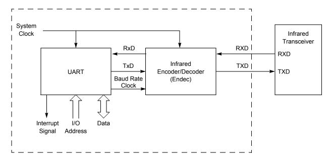
Figure 16. Infrared Data Communication System Block Diagram
