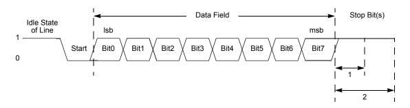
Figure 11. UART Asynchronous Data Format without Parity
