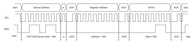
Figure 1: I<sup>2</sup>C Serial Interface Diagram.
