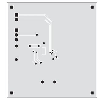
Figure 11: AAT1236 Evaluation Board Bottom Side Layout.
