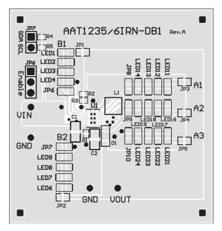
Figure 10: AAT1236 Evaluation Board Top Side Layout.
