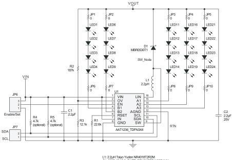
L1: 2.2µH Taiyo Yuden NR4018T2R2M C1: 0805 10V 2.2µF X7R GRM21BR71A225KA01 C2: 0805 25V 2.2µF X7R GRM21BR71E225KA73L LED1-24: OSRAM LW M673 or equivalent
