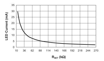
Figure 7: LED Current vs. R<sub>SET</sub> Values.
