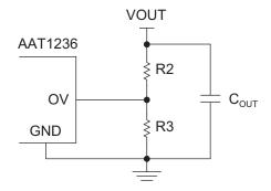
Figure 9: Over-Voltage Protection Circuit.
