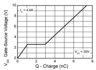
Gate-Source Voltage v Gate Charge
