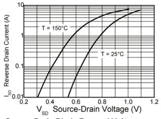
Source-Drain Diode Forward Voltage
