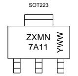
ZXMN 7A11 = Product Type Marking Code YWW = Date Code Marking Y or  $\overline{Y}$  = Last Digit of Year (ex: 5= 2015) WW or  $\overline{W}W$  = Week Code (01~53)
