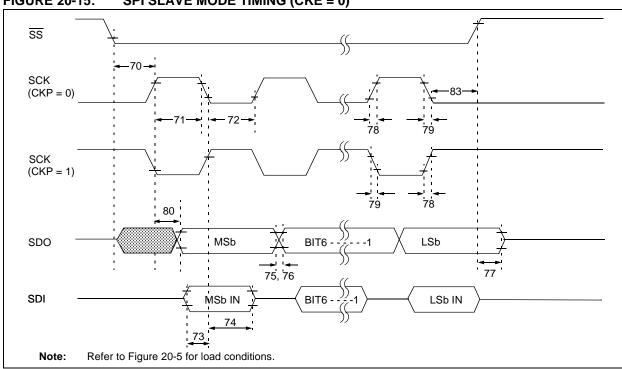
FIGURE 20-15: SPI SLAVE MODE TIMING (CKE = 0)
