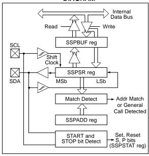
FIGURE 15-3: I<sup>2</sup>C MASTER MODE BLOCK DIAGRAM
