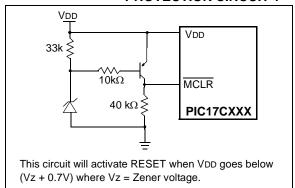
FIGURE 5-9: EXTERNAL BROWN-OUT PROTECTION CIRCUIT 2
