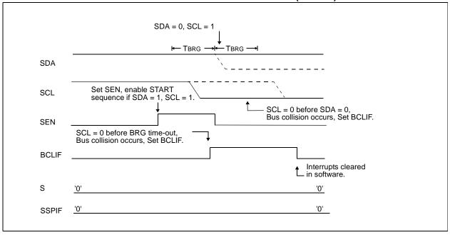
FIGURE 15-37: BRG RESET DUE TO SDA COLLISION DURING START CONDITION
