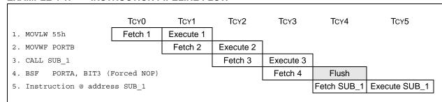
All instructions are single cycle, except for any program branches. These take two cycles since the fetched instruction is "flushed" from the pipeline, while the new instruction is being fetched and then executed.
