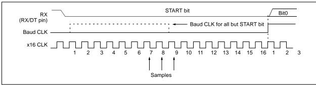
FIGURE 14-6: START BIT DETECT
