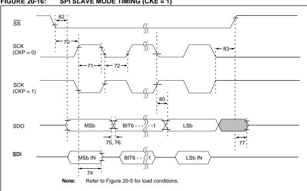
FIGURE 20-16: SPI SLAVE MODE TIMING (CKE = 1)
