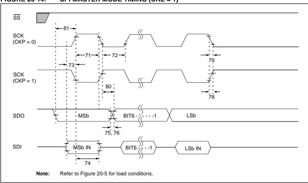
FIGURE 20-14: SPI MASTER MODE TIMING (CKE = 1)
