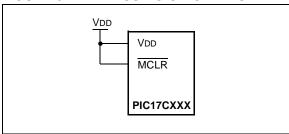
FIGURE 5-3: EXTERNAL POWER-ON RESET CIRCUIT (FOR SLOW VDD POWER-UP)
