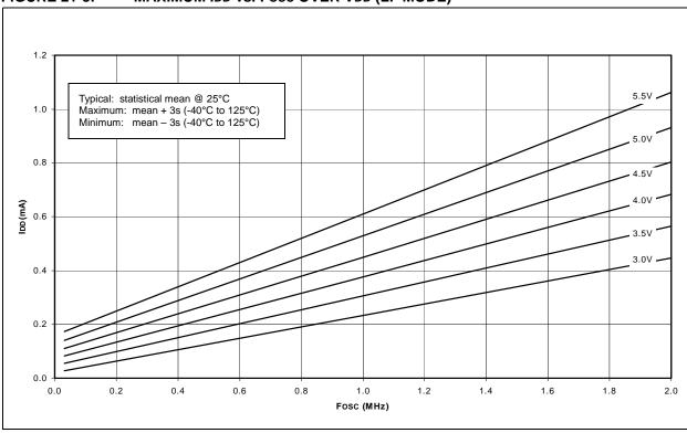
FIGURE 21-9: TYPICAL IDD vs. Fosc OVER VDD (XT MODE)
