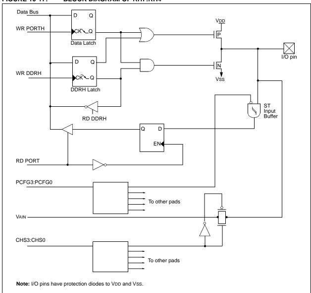
FIGURE 10-18: RH3:RH0 BLOCK DIAGRAM
