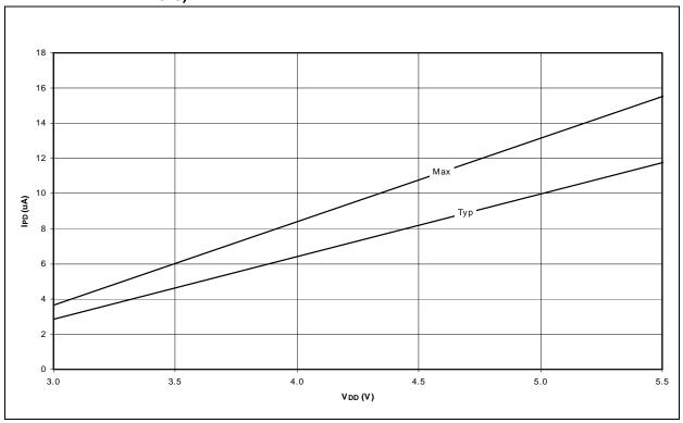
FIGURE 21-14: TYPICAL AND MAXIMUM AIRBPU vs. VDD (MEASURED PER INPUT PIN, -40°C TO +125°C)
