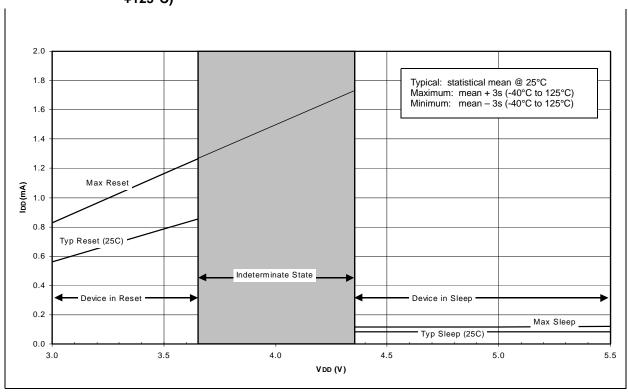
FIGURE 21-13: TYPICAL AND MAXIMUM  $\triangle$ IPD vs. VDD (SLEEP MODE, WDT ENABLED, -40°C to +125°C)
