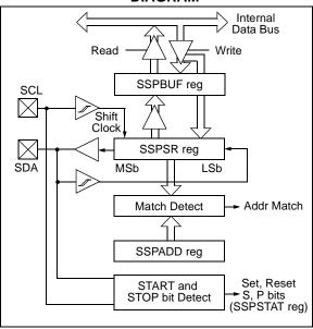
FIGURE 15-11: I<sup>2</sup>C MASTER MODE BLOCK DIAGRAM
