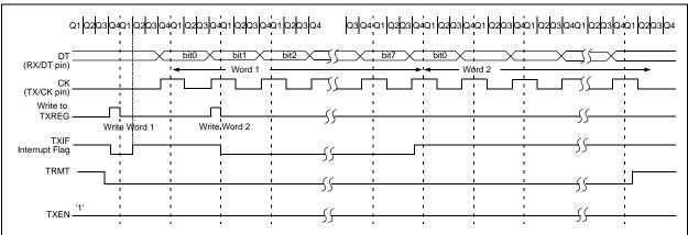
FIGURE 14-9: SYNCHRONOUS TRANSMISSION (THROUGH TXEN)
