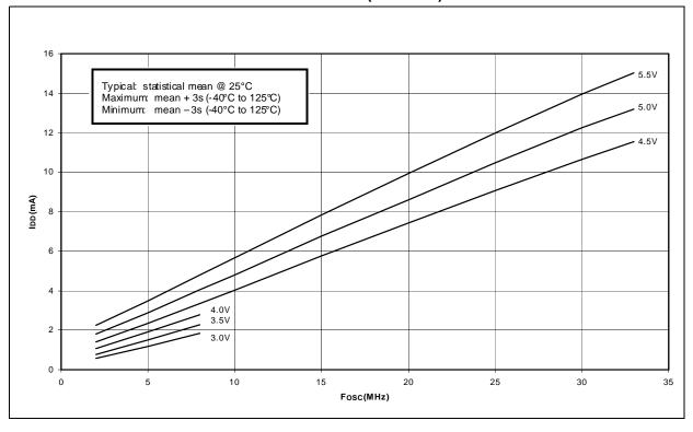
FIGURE 21-10: MAXIMUM IDD vs. FOSC OVER VDD (XT MODE)
