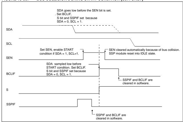
FIGURE 15-36: BUS COLLISION DURING START CONDITION (SCL = 0)
