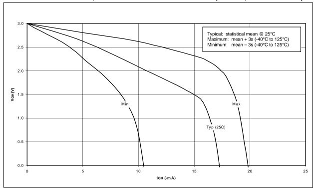
FIGURE 21-20: TYPICAL, MINIMUM AND MAXIMUM Vol vs. Iol (VDD = 3V, -40°C TO +125°C)
