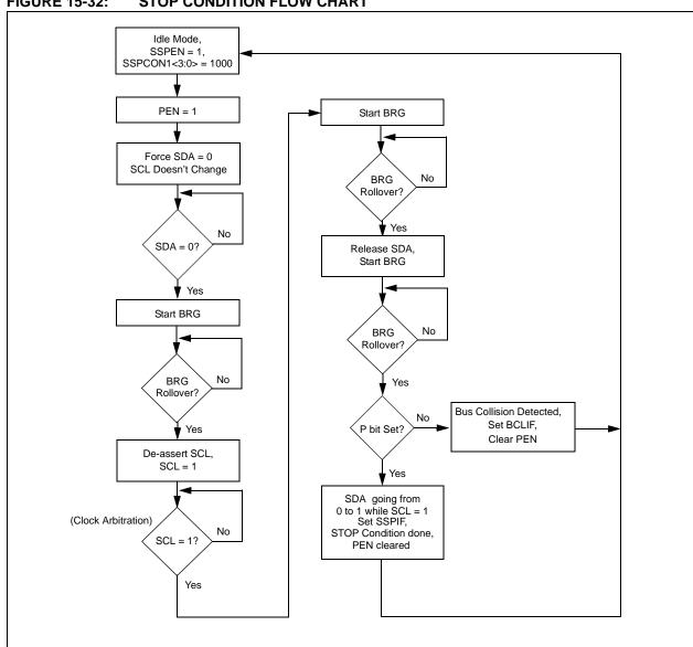
FIGURE 15-32: STOP CONDITION FLOW CHART
