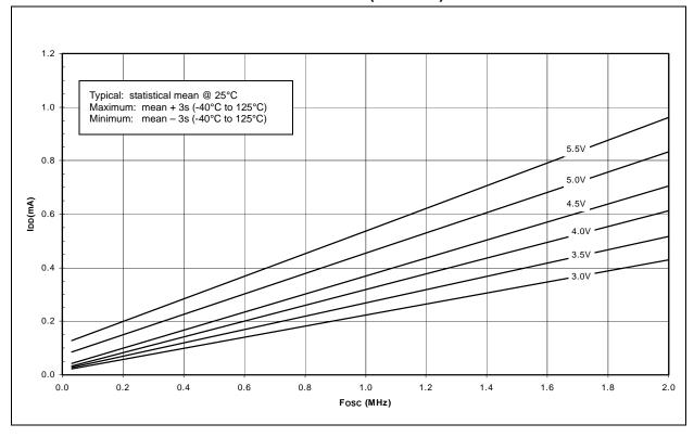
FIGURE 21-8: MAXIMUM IDD vs. Fosc OVER VDD (LF MODE)
