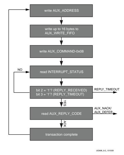
Figure 8-2: AUX Write Transaction
