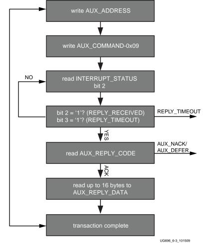
Figure 8-3 shows a flow of an AUX read transaction.
