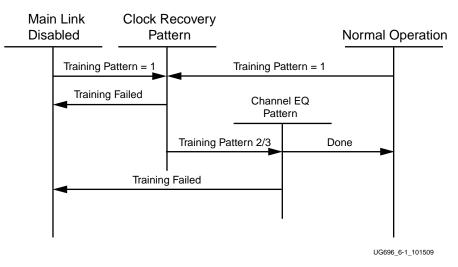
Figure 8-1 shows the flow diagram for link training.
