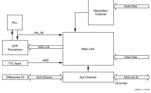
Figure 5-1: Source Core Top Level
