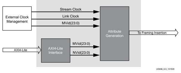
Figure 8-5: Transmitter Clock Generation
