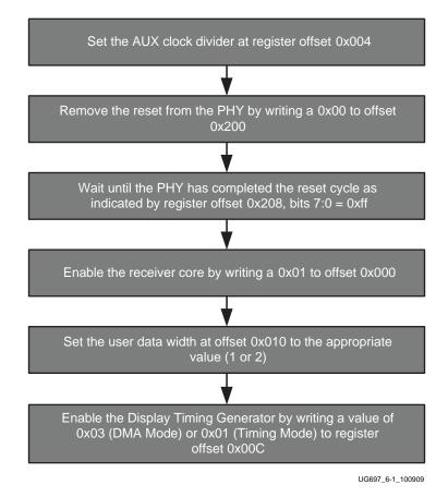
Figure 12-1: Receiver Core Initialization
