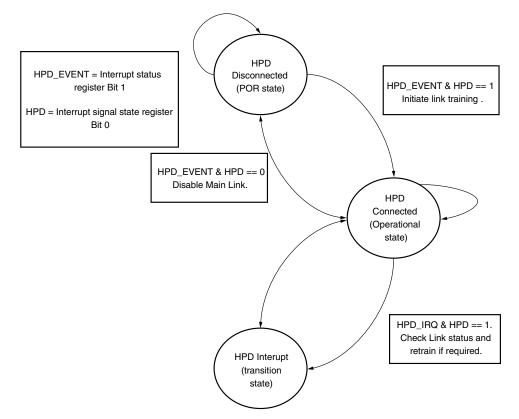
Figure 8-6: HPD Event Handling in Source Core
