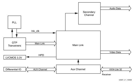
Figure 9-1: Sink Core Top Level
