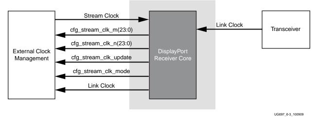
Figure 12-3: Receiver Clock Generation
