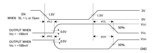
Figure 12. Receiver 3-STATE Delay Waveforms
