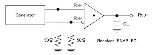
Figure 9. Receiver Propagation Delay and Transition Time Test Circuit
