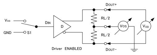
Figure 4. Driver VOD and VOS Test Circuit
