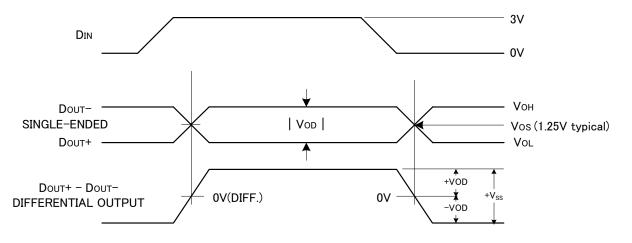
Figure 14. Driver Output Levels
