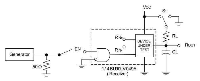
Figure 11. Receiver 3-STATE Delay Test Circuit
