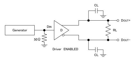
Figure 5. Driver Propagation Delay and Transition Time Test Circuit
