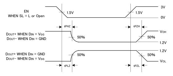
Figure 8. Driver 3-STATE Delay Waveform
