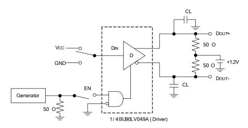
Figure 7. Driver 3-STATE Delay Test Circuit
