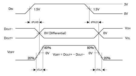
Figure 6. Driver Propagation Delay and Transition Time Waveforms
