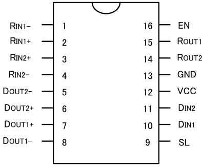
Figure 3. Pin Diagram (Top View)
