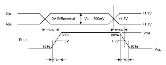
Figure 10. Receiver Propagation Delay and Transition Time Waveforms
