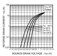
Fig.9 Reverse Drain Current vs. Source-Drain Voltage
