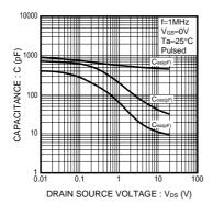
Fig.10 Typical Capacitance vs. Drain-Source Voltage
