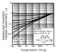
Fig.14 Normalized Transient Thermal Resistance vs. Pulse Width
