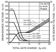
Fig.11 Dynamic Input Characteristics
