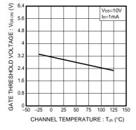
Fig.4 Gate Threshold Voltage vs. Channel Temperature
