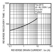
Fig.12 Reverse Recovery Time vs. Reverse Drain Current
