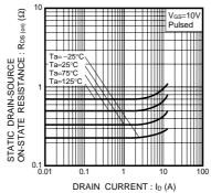
Fig.5 Static Drain-Source On-State Resistance vs. Drain Current
