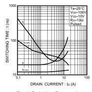
Fig.13 Switching Characteristcs
