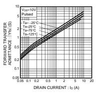
Fig.8 Forward Transfer Admittance vs. Drain Current
