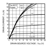
Fig.2 Typical Output Characteristics
