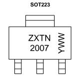
ZXTN 2007 = Product Type Marking Code YWW = Date Code Marking Y or  $\overline{Y}$  = Last Digit of Year (ex: 5 = 2015) WW or  $\overline{W}W$  = Week Code (01 - 53)
