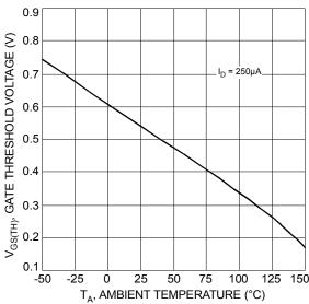
Fig. 5 Gate Threshold Variation vs. Ambient Temperature
