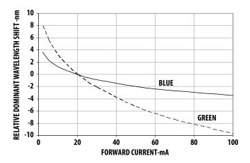
Figure 9. Relative dominant wavelength vs Forward Current
