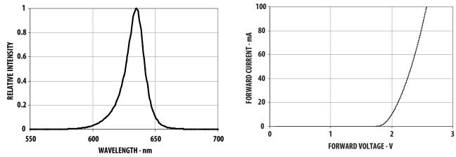
Figure 1. Relative Intensity vs Wavelength
