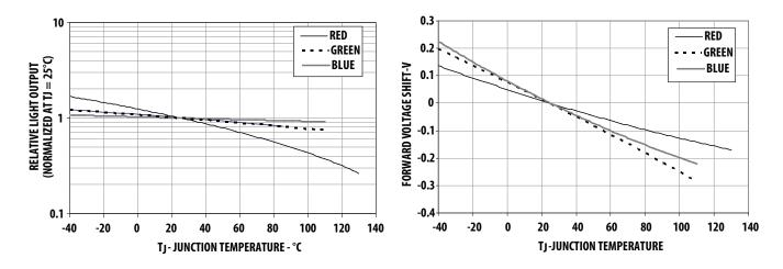
Figure 12. Relative Light Output vs Junction Temperature
