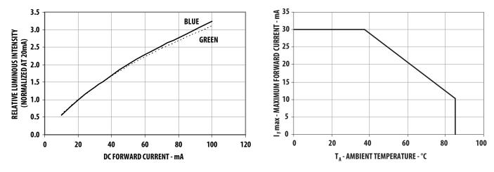
Figure 7. Relative Intensity vs Forward Current
