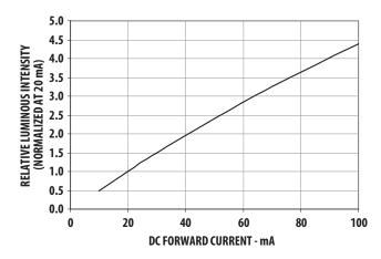
Figure 3. Relative Intensity vs Forward Current
