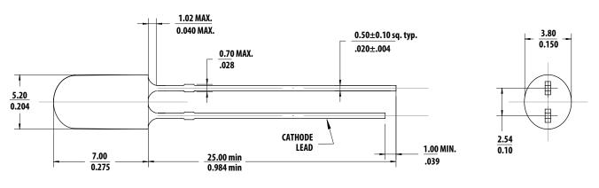
Notes: All dimensions in millimeters (inches). Tolerance is  $\pm$  0.20mm unless other specified
