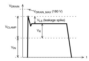
Figure 44. Power Switch Waveforms with Clamping
