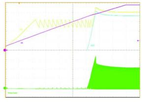
Figure 5. Startup Sequence,  $R_{CL}$  Open, Output Load = 80  $\Omega$  (I<sub>OUT</sub> = 150 mA), 1 V<sub>CC</sub> 3.0 V/ div DC, 2 V<sub>OUT</sub> 3.0 V/div DC, 3 V<sub>IN</sub> 10.0 V/ div DC, 4 I<sub>PRI</sub> 100 mA/div DC, T = 20 ms/div
