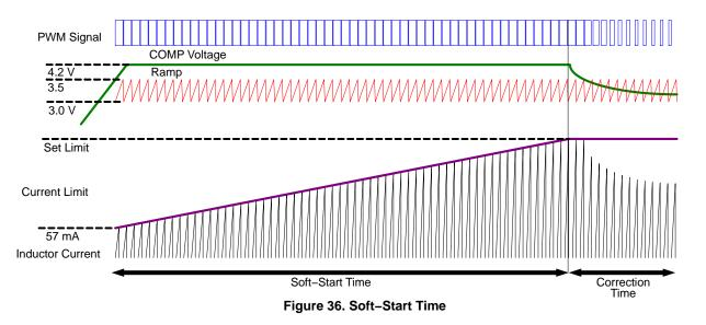
The compensation of the converter must be manipulated to minimize the overshoot of the output voltage during startup, details are in the compensation section.
