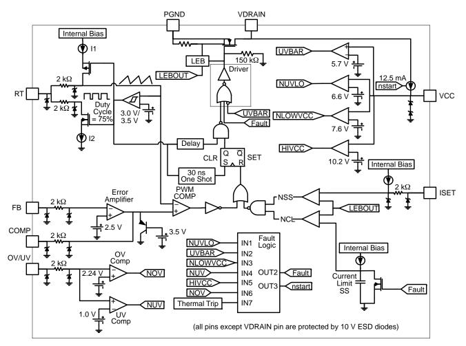
Figure 2. NCP1032 Simplified Block Diagram
