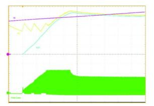
Figure 7. Soft–Start,  $R_{CL} = 32 \text{ k}\Omega \text{ (C}_{LIM} = 250 \text{ mA})$ , Output Load = 240  $\Omega \text{ (I}_{OUT} = 50 \text{ mA})$ , 1 V<sub>CC</sub> 3.0 V/div DC, 2 V<sub>OUT</sub> 3.0 V/div DC, 3 V<sub>IN</sub> 10.0 V/div DC, 4 I<sub>PRI</sub> 100 mA/div DC, T = 1.0 ms/div
