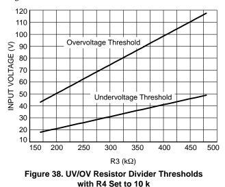
The UV/OV pin can also be used to implement a remote enable/disable function. If an external transistor pulls the UV/OV pin below 1.0 V (or above 2.4 V) the converter will be disabled and no switching is allowed. A device version is available without the OV protection feature, see the ordering
