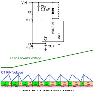
Figure 41. Voltage Feed Forward
