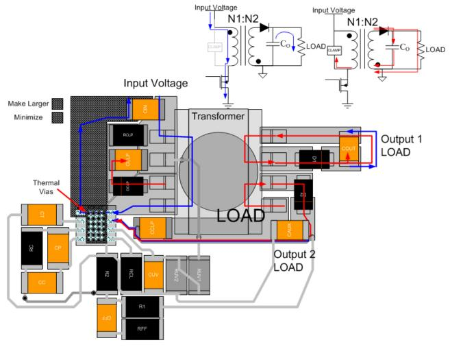
Figure 48. Recommended PCB Layout
