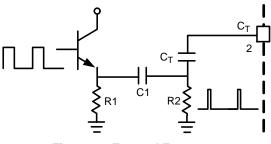
Figure 40. External Frequency Synchronization Circuit
