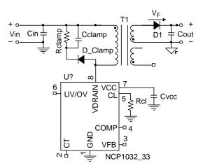
Figure 45. Passive RCD Clamp Network
