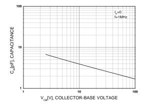
Figure 1. Feedback Capacitance
