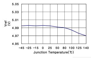
Figure 3. Trimmed Reference Voltage
