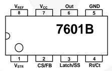
Figure 2. Pin Assignments (Top View)
