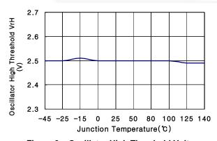
Figure 9. Oscillator High Threshold Voltage
