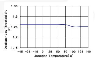
Figure 10. Oscillator Low Threshold Voltage
