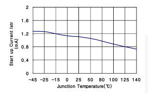
Figure 11. Startup Current
