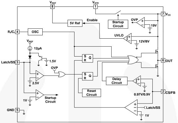
Figure 1. Internal Block Diagram
