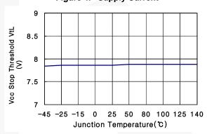
Figure 6. V<sub>CC</sub> Stop Threshold Voltage
