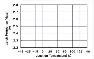
Figure 13. Latch Protection Voltage
