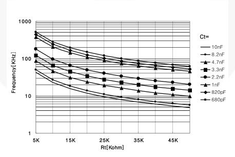
Figure 15. Oscillator Frequency Characteristic
