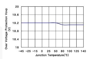
Figure 12. Over-Voltage Protection Level
