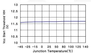
Figure 5. V<sub>CC</sub> Start Threshold Voltage
