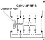
Note: Check carefully the coil polarity of the Relay.
