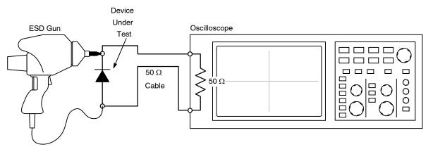
Figure 7. Diagram of ESD Test Setup
