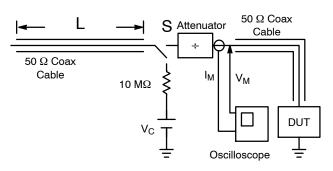
Figure 4. Simplified Schematic of a Typical TLP System
