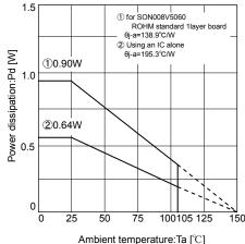
Fig.95 Thermal derating curve (SON008V5060)
