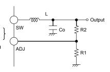
Fig.102 Determination of output voltage
