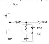
Output capacitor should be selected with the consideration on the stability region and the equivalent series resistance required to smooth ripple voltage. Output ripple voltage is determined by the equation (4):
