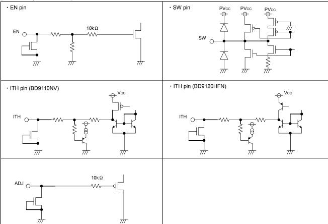
Fig.105 I/O equivalence circuit
