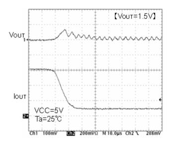
Fig.39 Transient response Io=600→100mA(10µs)
