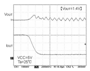
Fig.69 Transient response Io=600→100mA(10µs)
