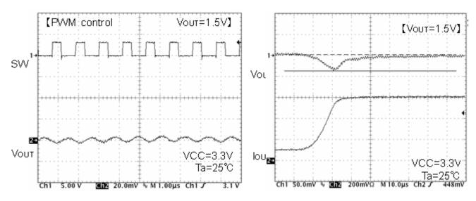
Fig.82 SW waveform Io=200mA
