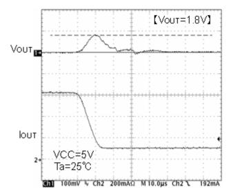
Fig.24 Transient response Io=600→100mA(10µs)
