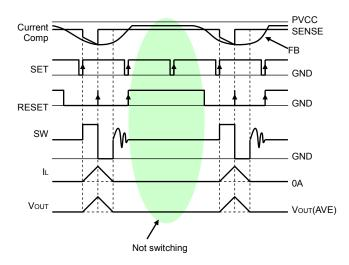
Fig.87 SLLM switching timing chart
