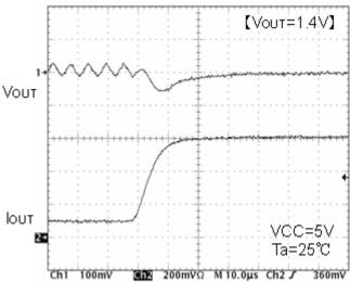
Fig.67 SW waveform Io=500mA
