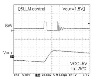
Fig.36 SW waveform Io=10mA
