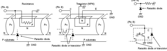
Fig.106 Simplified structure of monorisic IC
