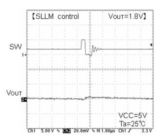
Fig.20 Soft start waveform
