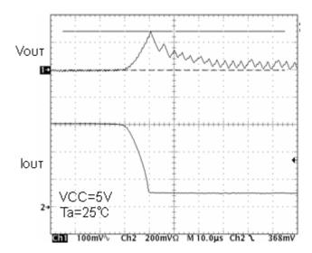
Fig.54 Transient response Io=600→100mA(10µs)
