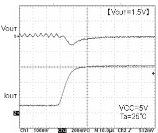
Fig.37 SW waveform Io=500mA
