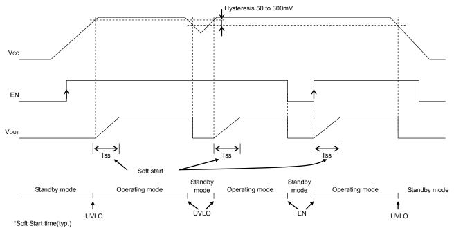
Fig.88 Soft start, Shutdown, UVLO timing chart
