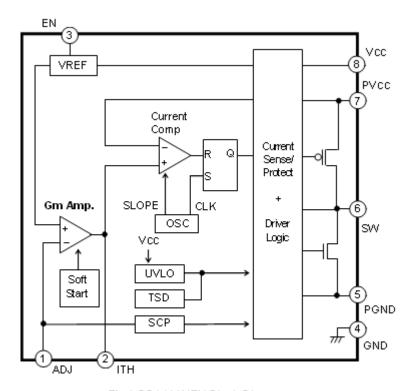
Fig.9 BD9120HFN Block Diagram
