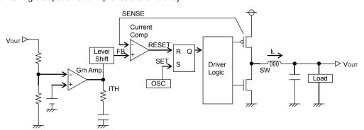
Fig.85 Diagram of current mode PWM control
