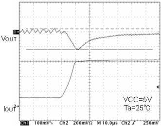
Fig.52 SW waveform Io=500mA
