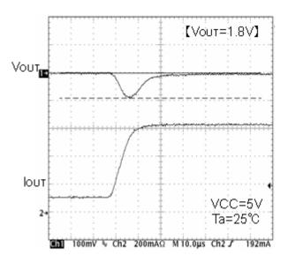
Fig. 23 Transient response Io=100→600mA(10µs)
