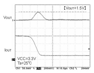
Fig.84 Transient response Io=600→100mA(10μs)
