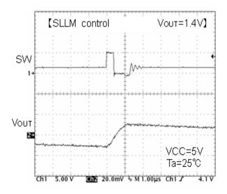
Fig.66 SW waveform Io=10mA
