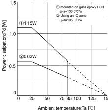
Fig.94 Thermal derating curve (HSON8)
