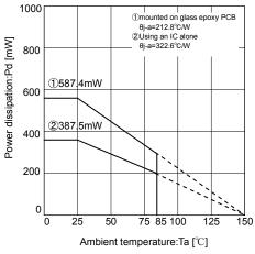
Fig.93 Thermal derating curve (MSOP8)
