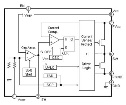
Fig.7 BD9109FVM Block Diagram
