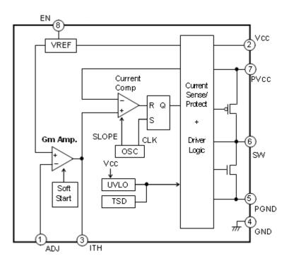
Fig.8 BD9110NV Block Diagram
