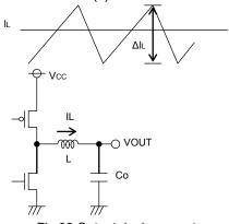
Fig.96 Output ripple current
