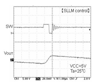
Fig.51 SW waveform Io=10mA
