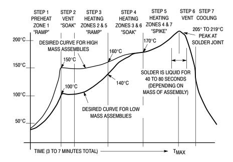
Figure 5. Typical Solder Heating Profile
