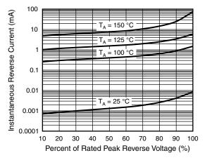
Fig. 4 - Typical Reverse Characteristics
