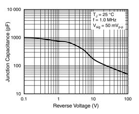
Fig. 5 - Typical Junction Capacitance
