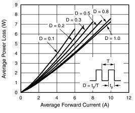
Fig. 2 - Forward Power Loss Characteristics
