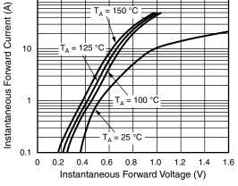
Fig. 3 - Typical Instantaneous Forward Characteristics
