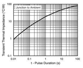
Fig. 6 - Typical Transient Thermal Impedance
