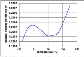
FIGURE 2-9: Internal Voltage Reference vs. Temperature.
