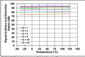
FIGURE 2-7: SINAD vs. Temperature.
