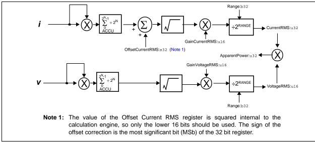
FIGURE 5-2: RMS Current and Voltage Calculation Signal Flow.
