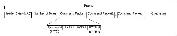
FIGURE 4-1: MCP39F501 Communication Frame.
