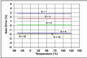
FIGURE 2-8: Gain Error vs. Temperature.
