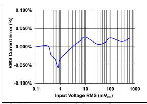
FIGURE 2-2: RMS Current, Gain = 1.
