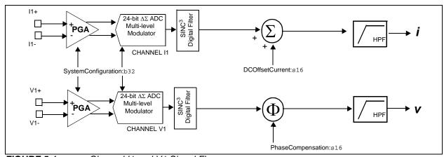
FIGURE 5-1: Channel I1 and V1 Signal Flow.
