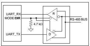
FIGURE 4-2: DIR Pin Operation Using Example RS-485 Bus Transceiver.
