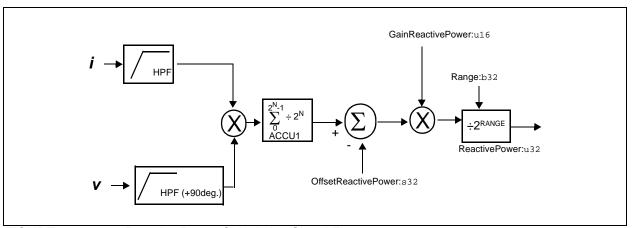
FIGURE 5-4: Reactive Power Calculation Signal Flow.
