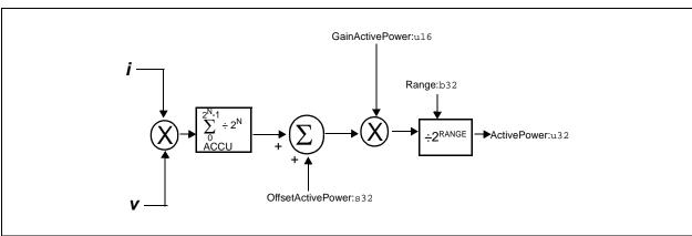
FIGURE 5-3: Active Power Calculation Signal Flow.
